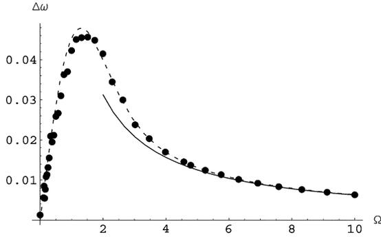
Fig. 1. Frequency deviation  $\Delta\omega$  as a function of the oscillator frequency  $\Omega$ , with noise level  $\kappa = .25\tau^{-1}$ , calculated from the phase mean over  $10^4$  realizations. The correlation function of the noise sources is given by (7). The dotted line is determined from the approximation (38); the line is the asymptotic power law (46). The frequency  $\Omega$  and the mean frequency are expressed in units of  $\tau^{-1}$ .
