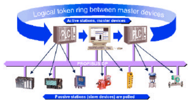
Fig 1: Master-Slave Communications in PROFIBUS
